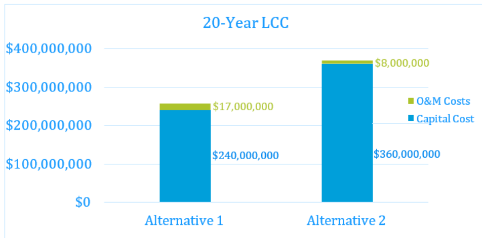
Figure 4-1 Life Cycle Cost for the Two De Pere Facility Alternatives
