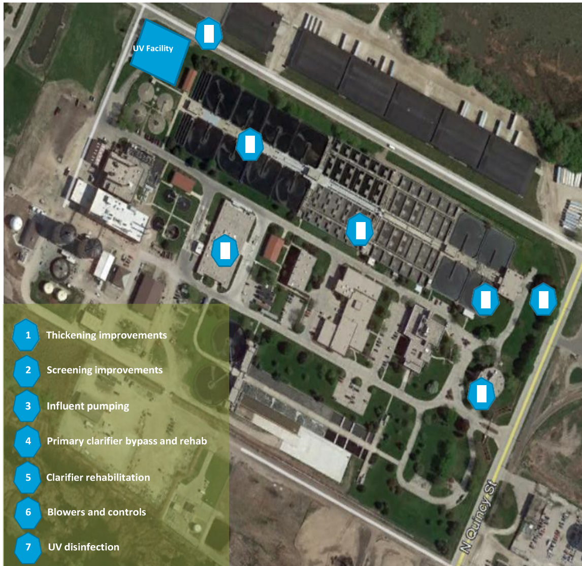
Figure 3-2 Alternative 1 Green Bay Facility Recommended Improvements
