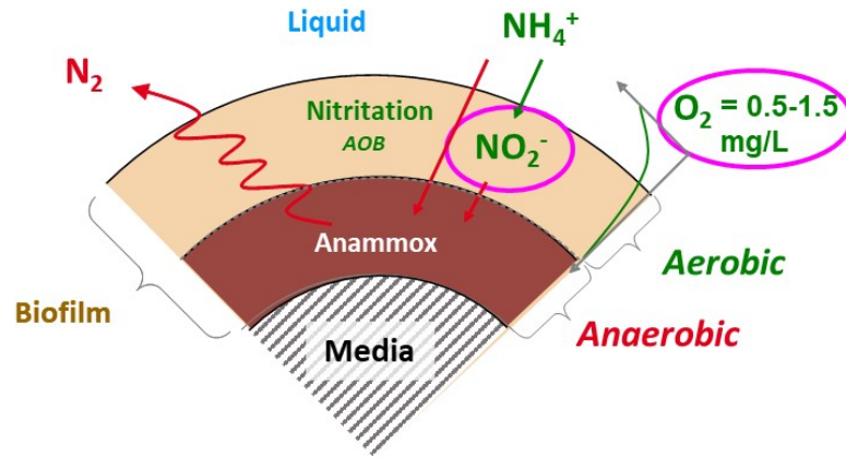
Figure 5-2 Depiction of Bacterial Populations Attached to ANITA Mox Media Carriers for MMBR Configurations. Image (Image Courtesy of Veolia)
