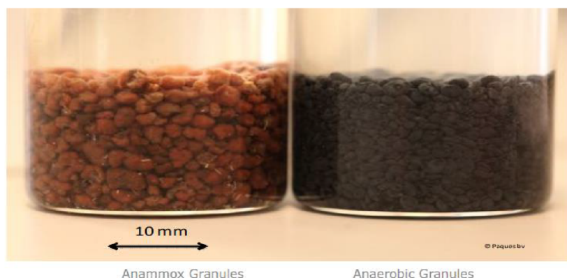
Figure 5-5 AnammoPAQ Anammox Granule Comparison to Anaerobic Granules (Image Courtesy of Ovivo)
