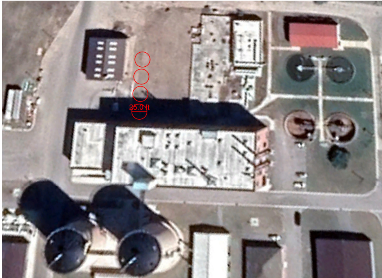
Figure 3-2 Proposed Location for Dewatered Sludge Cake Silos
