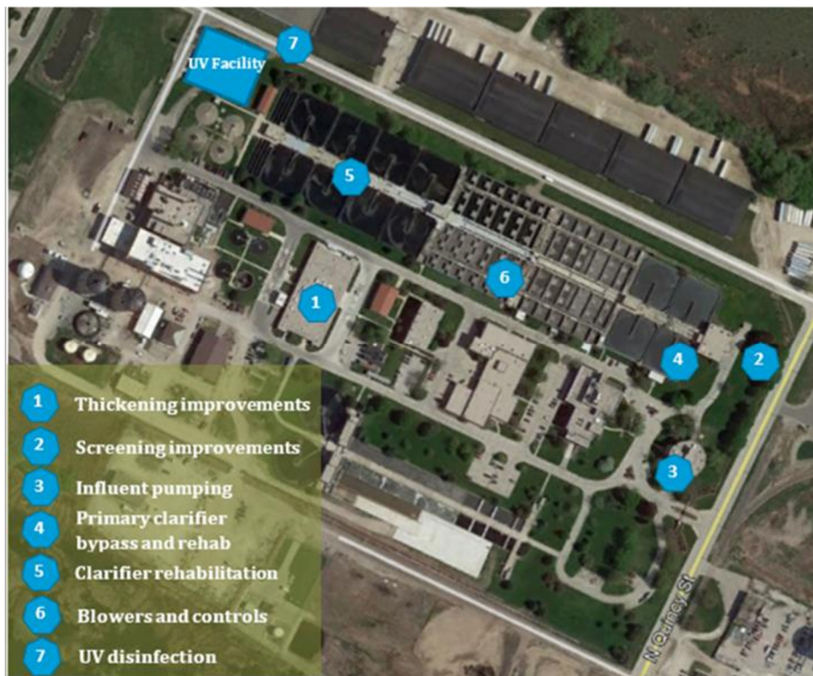
Figure 6-2 Alternative 1 Green Bay Facility Recommended Improvements
