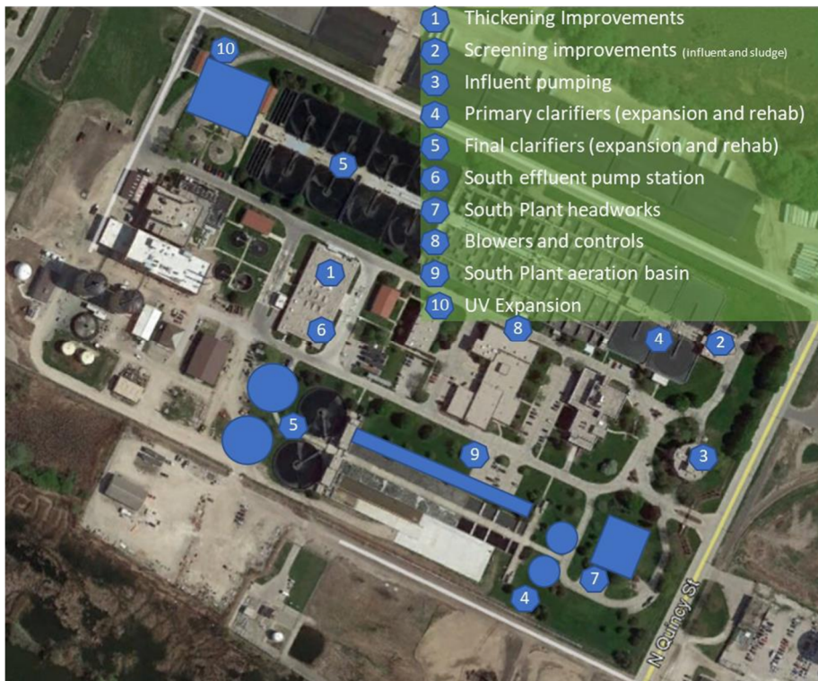
Figure 6-4 Alternative 2 Green Bay Facility Recommended Improvements
